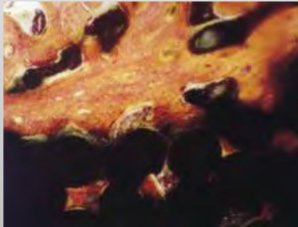
Magnification of Porocoat Porous Coating
